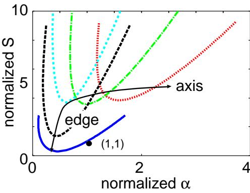
Beta limit increased with edge pressure gradient.
